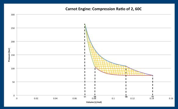
Figure 2: Carnot Cycle on P-V Plot
