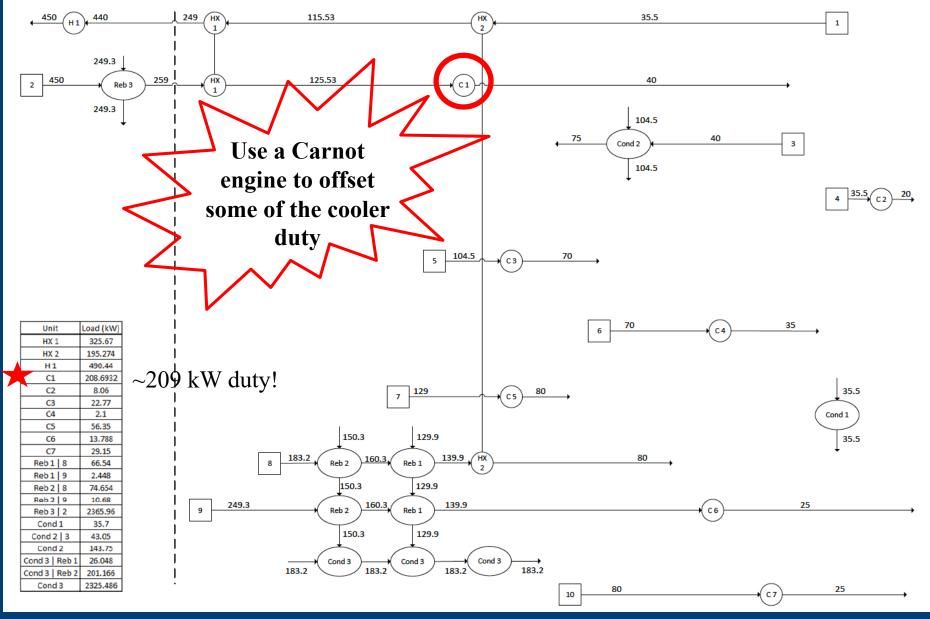
Figure 5: Toluene Process- Streams Diagram
